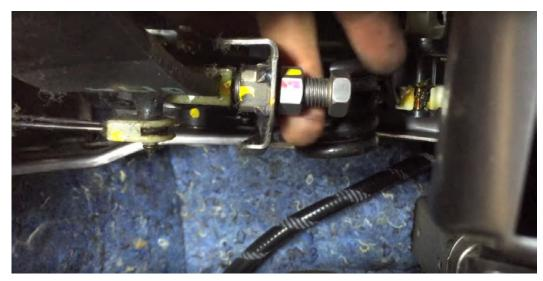
3) Adjust the pushrod from the master cylinder to the pedal by undoing the locking nut and rotating the pushrod. This must have a small amount of freeplay when wriggled by hand. This is to ensure that there is no excess pressure on the master cylinder. Failure to do so could cause the clutch to prematurely slip. Tighten the locking nut to ensure that the pushrod does not adjust as the clutch is operated.
